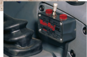
Coupler switch is within easy reach of operator's seat
